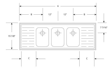
Note: For counter cut out, subtract 2 5/8" from length and depth dimensions.
